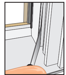
Pry off Monumental Double-Hung jamb liner
