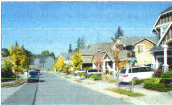
This relatively flat street is on a site with a 15% cross slope. Grade is taken up through buildings and rear lot rockeries. The flat street provides a good walking environment and usable common outdoor space, and helps unite the neighborhood.
