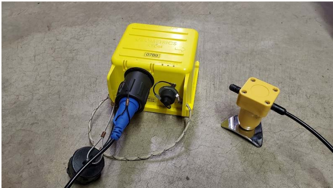
Figure 2. Seismograph and Geophone
