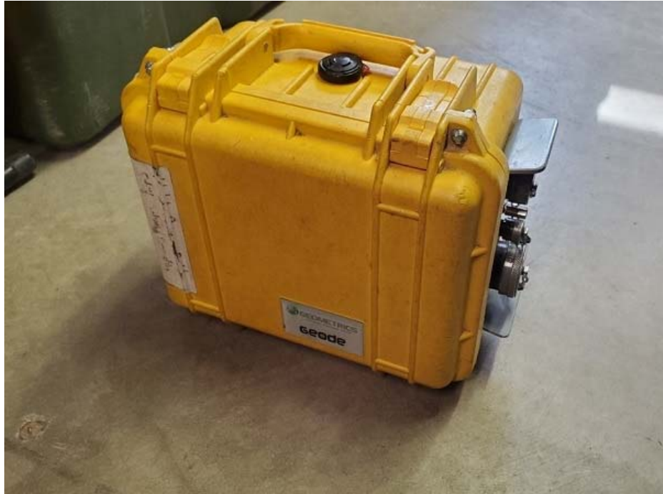
Figure 3. Geometrics Geode Seismograph
