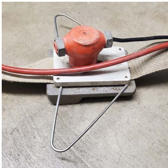
Figure 4. Land streamer geophone
